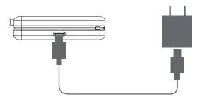
Type-C Cable Connection (Charging the power bank)
